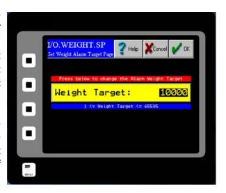
Step 7: Now return to the I/O.ALARM.SP page by pressing the OK Button in the upper right hand corner of the screen. You must now choose which type of Weight Output you would like to utilize. Press the WEIGHT OUTPUT Button for your options. You should now be on the I/O.WEIGHT.OUT page. More information on the two types of Weight Output, Pulse and Latch, can be found on the I/O.WEIGHT.OUT page in the Screen Guide section of the manual.
